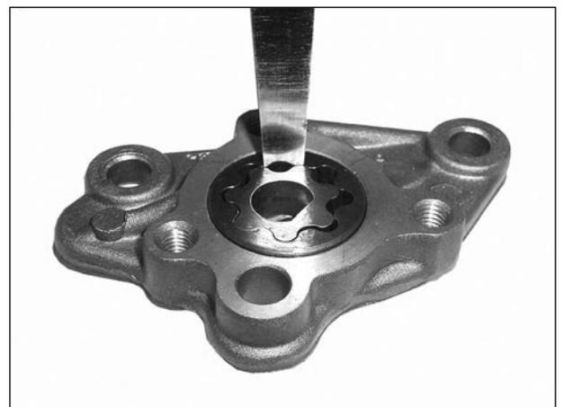
Measure the pump body clearance.
